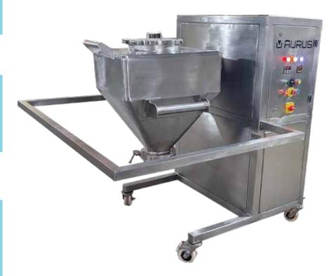
Charging hole with hinged lid with seal for charging and cleaning.
